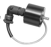
provide smooth control of unwind stands operating at any speed. The sensor is mounted at one end of the dancer roll pivot shaft where it monitors the angular position, direction of travel and relative speed of dancer arm movement. TCS-605-2 used with drive systems.
