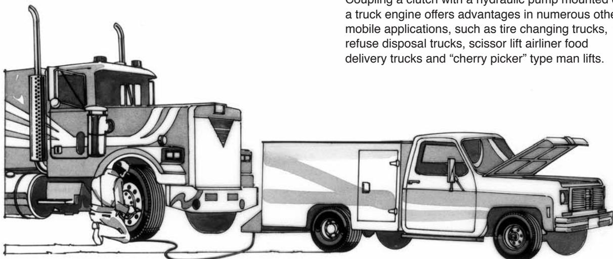
Coupling a clutch with a hydraulic pump mounted on a truck engine offers advantages in numerous other mobile applications, such as tire changing trucks, refuse disposal trucks, scissor lift airliner food delivery trucks and “cherry picker” type man lifts.
