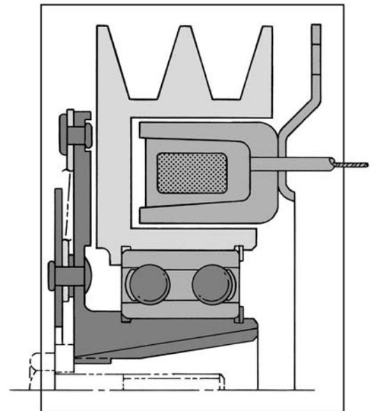
Electric clutches provide for remote control of the feed and chopping mechanisms on straw choppers, insulation blowers, and salt spreaders.
