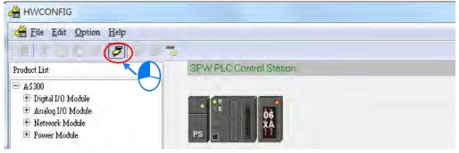
Generally speaking, a hardware configuration error occurs if the BUS FAULT LED indicator on the CPU module is ON. Users can select 06XA, click the right mouse button, and select **Diagnosis**.
