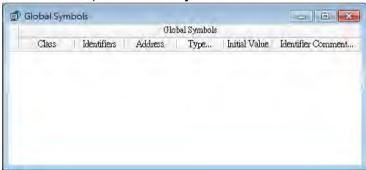
Double-click the blank to open the **Add Symbol** window. Type "X0.0" in the **Address** box. The default values in the **Type...** box, the **Initial** box, and the **Comment...** box remain unchanged. Click **OK** to complete the typing.
