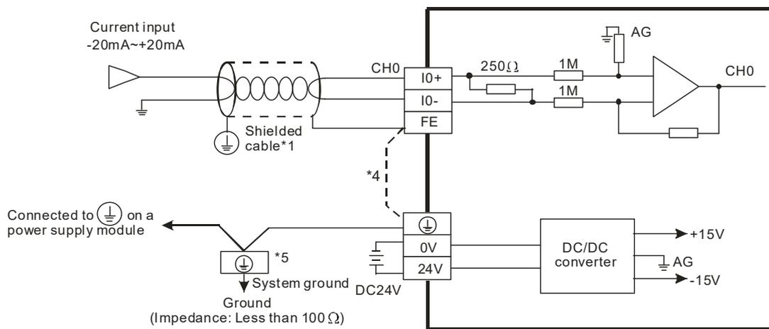
\*1: Please isolate analog input cables from other power cables.
