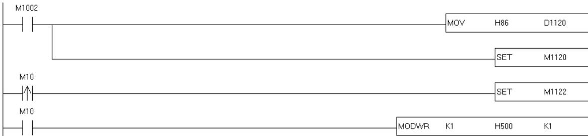
**Step 2:** Connect COM2 on TP70P-16TP1R to the two RS-485 wires connected to a DVP series PLC. When M10 is ON, Y0 on the DVP series PLC is ON.
