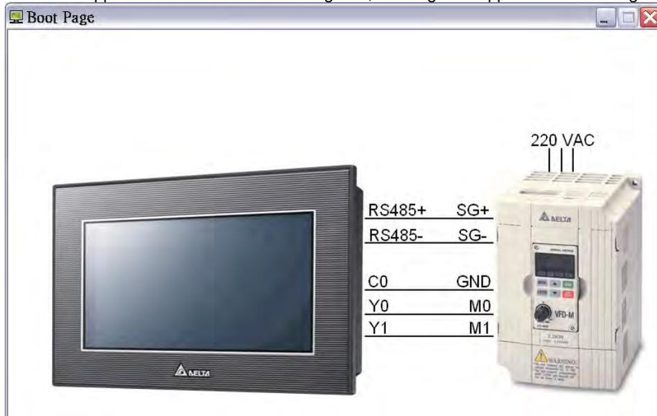
The state of the AC motor drive used is displayed on page 0, that is, the current rotational speed of the AC motor drive, a warning message, forward rotation control, backward rotation control, and stop control are displayed on page 0.
