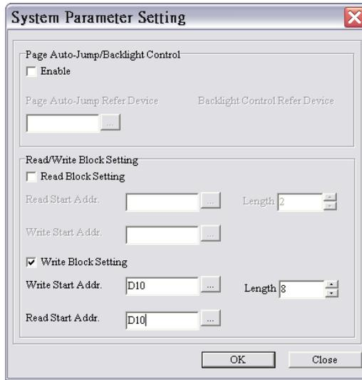
**Step 2:** Click **...** at the right side of the **Write Start Addr.** box. Select the **External PLC Setting** option button and D10 in the **Refer Device** window.
