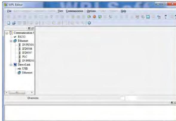
Step 2: After
