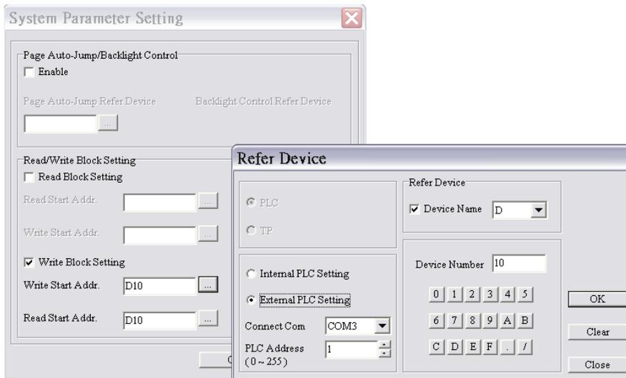
**Step 3:** After the steps above are complete, and the program in TPEditor is downloaded to TP70P, TP70P can exchange data with the DVP PLC series by means of COM3.
