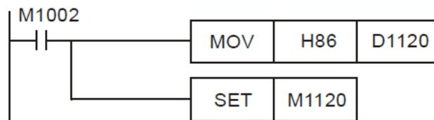
**Example: PLC communication uses an RTU mode.**
