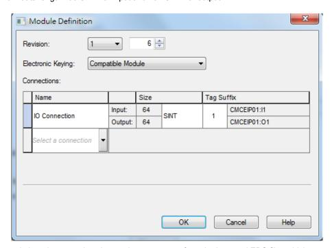
In general, there is no need to change the parameters from the imported EDS files which can usually be used without modification. • In the New Module dialog box, click the Connection tab to modify the Requested Packet Interval and Input Type settings. The RPI uses the I/O connection to a Scanner to exchange data at regular intervals, and the units are micro-seconds. For Input Type select either Unicast or Multicast. The Input Type selections may vary for different products.
