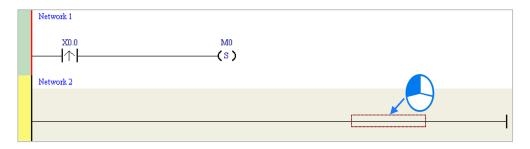
(2) Type the IL instruction "LD M0". This instruction is not case-sensitive. As soon as you type the IL instruction, a box which you can edit appears. After you finish typing the IL instruction, press Enter on the keyboard or click **OK** at the right side of the box.
