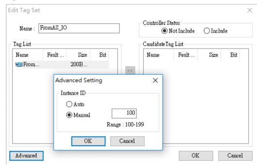
7. Use the same method to set the Instance ID manually for IDs in In-Consume section as you have set for IDs in Out-Produce section.
