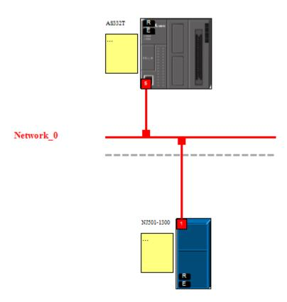
10. Right-click the CPU's communication port and select **Data Mapping** to create a data mapping table.
