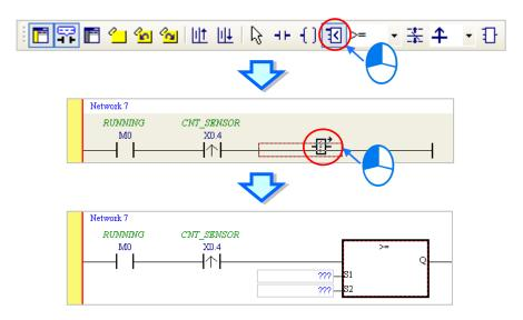
Write the program shown below. In ISPSoft, K precedes a decimal value and H precedes a hexadecimal value. To type a decimal value in ISPSoft, type it directly. To type a hexadecimal value in ISPSoft, type "16#" and the hexadecimal value; e.g. 16#7FFF. In ISPSoft, 8# precedes an octal value, and 2# precedes a binary value.
