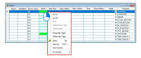
You can text and debug the program you created in this chapter through the monitoring table you created in this section. Refer to Chapter 18 in the ISPSoft User Manual for more information about testing and debugging a program.
