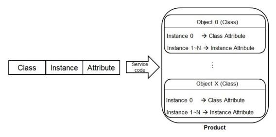
You can use API 2208 EIPRW instruction or explicit messages to read / write objects. The supported EtherNet/IP objects are listed in the following table. Refer to Section 9.8.2 for the data type definitions. Refer to Section  $9.8.3 \sim 9.8.19$  for object contents.
