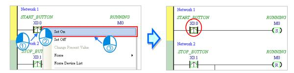
However, you can force an input contact ON or OFF during a test. Click an input or output contact to set, right-click the contact, point to **Force**, and click **On (X/Y)**, **Off (X/Y)**, **Release (X/Y)**, or **Release AII**. If you force an input or output contact ON or OFF, a lock symbol appears at the left side of the contact.
