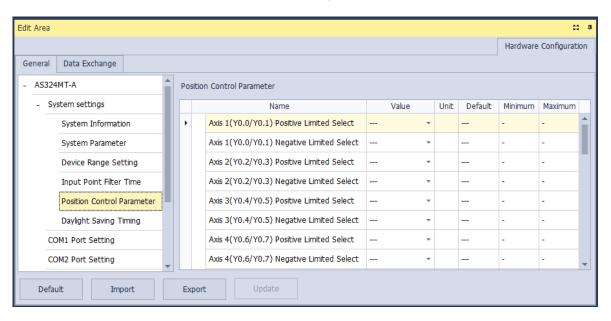
Axis1 (Y0.0/Y0.1) Positive/negative Limited Select ~ Axis 6 (Y0.10/Y0.11) Positive/negative Limited
