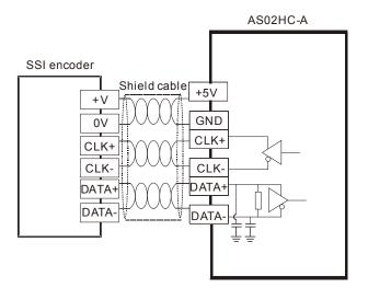
Note: The power supply of the SSI encoder you are using may NOT be 5 VDC, check for the actual power supply of your SSI encoder.
