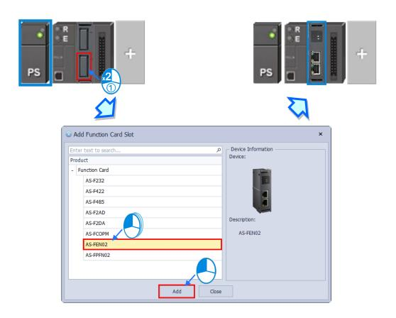
You can also set AS-FEN02 card in the Edit Area. Set AS-FEN02 as **Manual Select Card** (Note: If AS-FEN02 card is selected from **Manual Select Card**, then Function Card 1 cannot be set.) After that you can set up Ethernet communication parameters.
