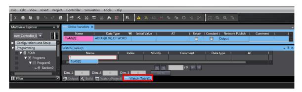
Modify the values according to the display format. Make sure the value in the **Online Value column** is the same as the value in the **Modify column**.
