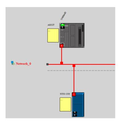
2. The solid network lines indicate the data mapping is being monitored successfully.
