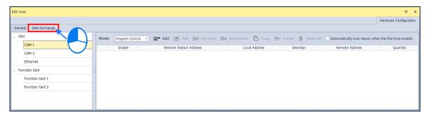
AS Series PLC CPU is built with two ports, two COM ports or one COM port and one Ethernet port varied by different models. When acted as a Master and performs data exchange with a remote Slave, the data exchange through COM1 and COM2 is via the Modbus protocol; if the data exchange through Ethernet is via the Modbus TCP protocol. The setting items for COM1, COM2 and Ethernet are the same.
