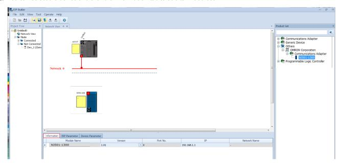
9. Drag and drop the red spare to have the Ethernet communication port connected to the network.
