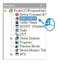
5. Save and download the settings from HWCONFIG: on the **File** menu click **Save** to save the settings and then click the download button on the toolbar to download the file to PLC. You must save the configuration in HWCONFIG before opening the other communication tools. While working in the communication tools, you cannot work in HWCONFIG.
