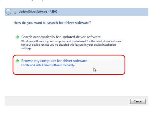
(4) After you install ISPSoft version 3.00 or later, the driver for the AS Series CPU module is under the folder where you installed ISPSoft ...\ISPSoft\drivers\Delta\_PLC\_USB\_Driver\. Enter the path to the driver, or click Browse to browse to the correct folder.
