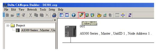
D. Click the Scan Network button on the Toolbar to scan the network.
