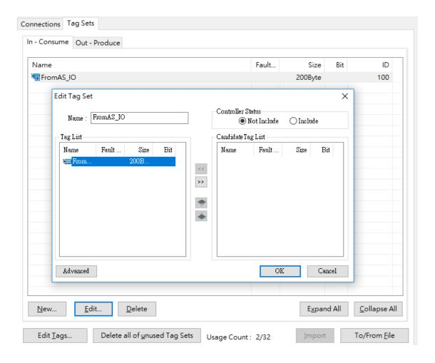
6. Click **Advanced** button in the Edit Tag Set window and set the Instance ID to **Manual** and then input the Instance ID you'd like to use for IDs in In-Consume section.
