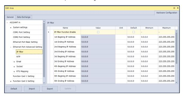
Select **IP Filter Function Enable** checkbox to enable the IP filter function and type the start address and end address of group 1~8 IP.
