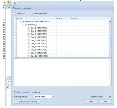
Step 3: Make sure you have the backup file ready and the IP addresses and Slave IDs in the backup file of the SD card are identical to the ones that need to be restored.
