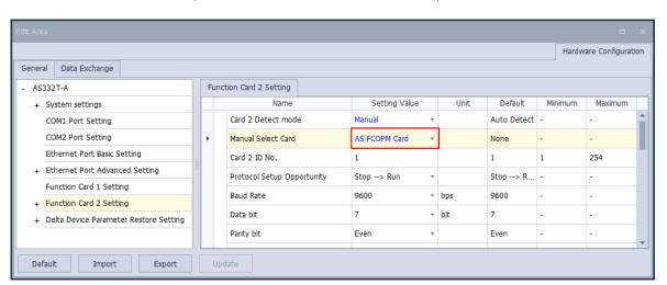
For AS-FCOPM Working mode, select AS Remote Communication, and then enter the number of the connected AS Remote module. Click Upate and then close the setting page.
