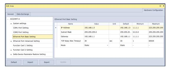
Mode sets the addressing mode of the IP of the CPU module.
