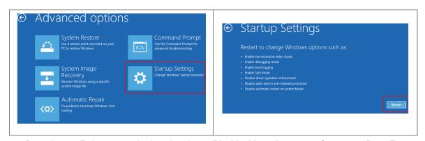
5. Press the 7 or F7 key on your keyboard to choose **Disable driver signature enforcement**. Press Enter and the system directs you back to the Windows 8 operating system. Install the Delta PLC USB driver now by connecting the AS Series CPU module to your computer's USB port. Refer to Section A2 for the steps to install the USB driver.
