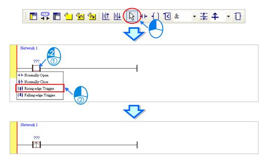
(3) Click the line at the right side of the contact, click on the toolbar, and then move the mouse cursor to the red frame. The mouse cursor changes to a coil when the mouse cursor is above or under the red frame. Decide where to insert the coil.
