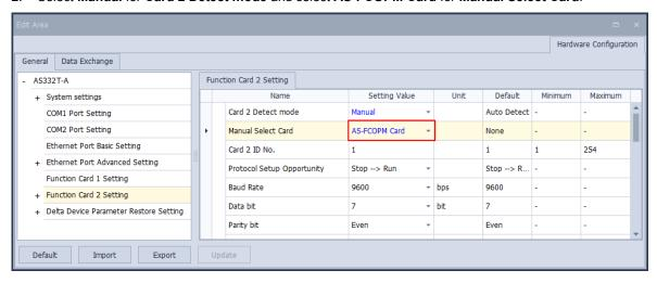
3. Select the working mode, node ID and the bit rate for AS-FCOPM.
