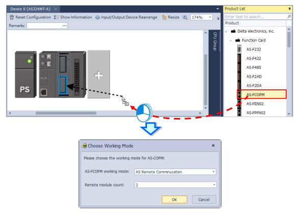
If you set the Remote module count to 2 and click OK, you can see two remote modules connected to the PLC CPU.
