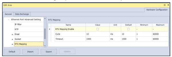
Select RTU Mapping Enable checkbox to enable the function of connection between RTU module and PLC CPU. Set the update cycle in **Cycle** box and a timeout in **Timeout** box. It means a timeout when RTU does not give a reply within the timeout set.
