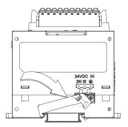
Use screws to secure the baffle.
