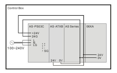
\*1. The live wire and the neutral wire in the AC power cable are connected to L and N on the power supply module respectively. To prevent incorrect system operation, the ground in the AC power cable must be connected to LG on the power supply module.
