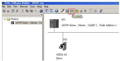
Note: you must reboot the AS300 Series PLC to enable the downloaded parameters.
