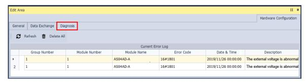
After you click Diagnosis, you can see a table with three tabs. On the Diagnosis tab, you can see the Current Error Log table. When the error is cleared, you can use to clear the error log stored in the module and the module state
