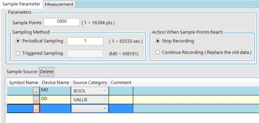
• Click the button of **Symbol Name** in the **Add Sample Source** window and select the variable symbol name to be added in the **Choose Symbol** window or directly type a device name in the **Device Name** box.
