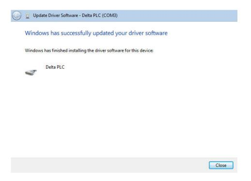
(7) Open the **Device Manager** window again. If the name of the Delta USB device appears under **Ports (COM & LPT)**, the installation of the driver is successful. The operating system assigns a communication port number to the USB device.
