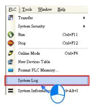
(2) The **System Log** window appears. Click **Clear Log** to clear the error log in the window and the error log in the CPU module, and reset the CPU module.
