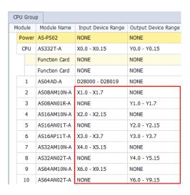
Note: though there is no information on the occupied data devices in the image shown above, the CPU reserves 20 words of data devices.
