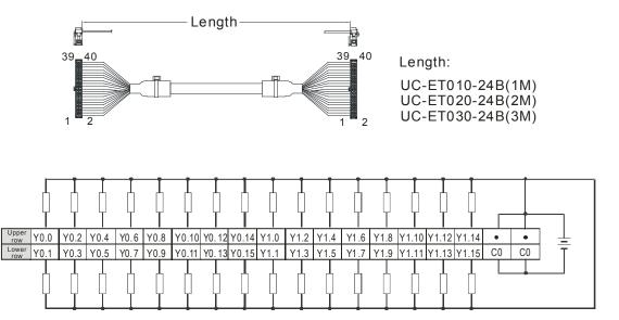
Note: UB-10-OT32A can be used with AS Series and DVP Series. The indications on the UB-10-OT32A board is for DVP Series. For the definitions of terminal connections for AS Series, you can see the reference table below. Or refer to the enclosed sticker for AS Series.
