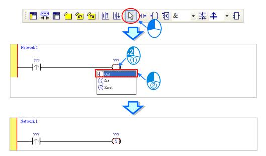
(5) Click ??? above the contact, type a device address in the box, and then press Enter on the keyboard to jump to the next box in the network. After you type a device address in the box, press Esc on the keyboard to complete the editing. In this example, type X0.0 in the box for the contact, and type M0 in the box for the coil.
