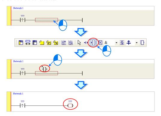
(4) Click on the toolbar, or press Esc on the keyboard. After you double-click the coil, a list appears.
