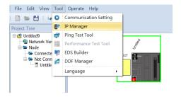
The IP Manager can be the BOOTP/DHCP Server, receiving IP address requests from devices. The IP Manager window is shown below.
