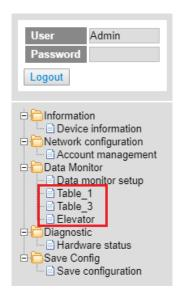
h. Note: The data monitor table must be downloaded to the device otherwise even if the data monitor table is created, it cannot be monitored.
