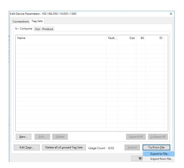
4. After the file is imported, make sure the input and output variables are imported in In-Consume and Out-Produce sections.
