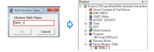
After you double-click the item, a item monitoring window appears. You can add items to be monitored to the window. To add an item to the window, double-click the blank space in the monitoring table, type a device name, type a start address, and the number of devices to be monitored in the **Device Monitor Input** dialog box. You can add up to 100 items to a monitoring table.
