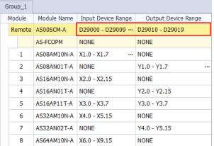
AS01DNET-A: when selecting the COM communication mode, its communication status and communication method: the input device range occupies 20 data registers, and the output device range occupies 20 data registers.
