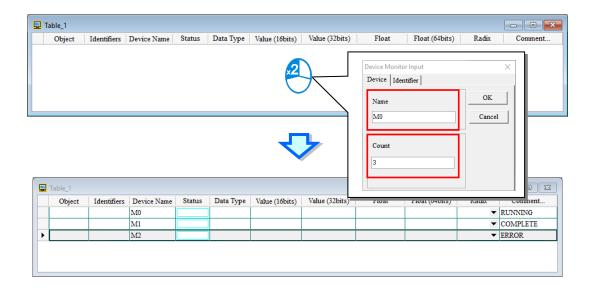
Press Insert on the keyboard to switch between inserting and replacing an item in the monitoring table. The selected mode displays in the status bar in ISPSoft.
