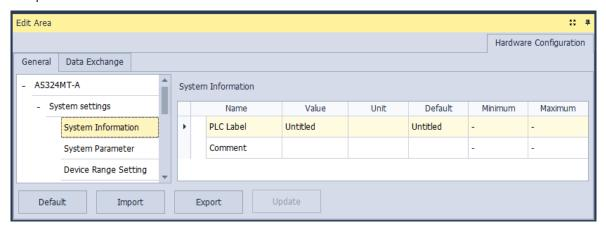
After the project is created, you can find the PLC label behind the product name in the project management area. You can change the PLC label in HWCONFIG as it is mentioned above. The PLC label is very useful when you have more than one PLC in the project. This label can be seen as the PLC identity. So that you will not change other PLC parameters by mistake. To prevent errors, when you download/upload the program, the system will remind you to check the name of the PLC CPU and the PLC label.
