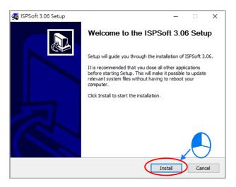
(6) The installation program detects if your computer has installed Microsoft Visual C++ 2013 or not. If not, the following installation steps will show up. Click **Install** to install and after the installation is done, click **Close**.
