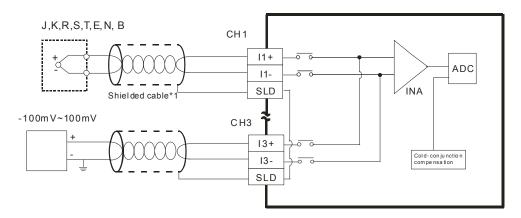
\*1. The cable connected to the input terminal should be the cable or the shielded twisted pair cable connected to a type J, K, R, S, T, E, N, B thermocouple. It should be kept separate from other power cables and cables that generate noise.
