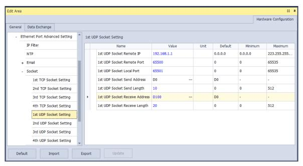
The parameters in the **TCP Socket Setting** are the same as the parameters in the **UDP Socket Setting** except that there is no **Keep Alive Timer** parameter in the UDP Socket Setting. The parameters in the TCP and UDP Socket Setting are described below.
