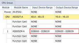
• Remote module SCM: the input device range and output device range each occupy 10 data registers.
