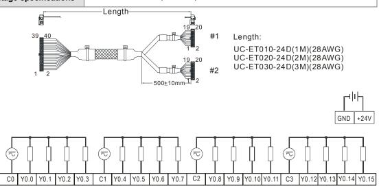
Note: UB-10-OR16A can be used with AS Series and DVP Series. The indications on the UB-10-OR16A board is for DVP Series. For the definitions of terminal connections for AS Series, you can see the reference table below. Or refer to the enclosed sticker for AS Series.
