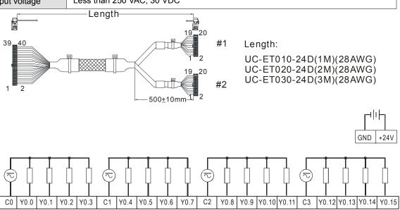
Note: UB-10-OR16A can be used with AS Series and DVP Series. The indications on the UB-10-OR16A board is for DVP Series. For the definitions of terminal connections for AS Series, you can see the reference table below. Or refer to the enclosed sticker for AS Series.
