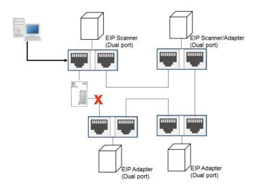
Alternatively, you can use an EIP tap to connect your PC so that the ring topology stays intact.
