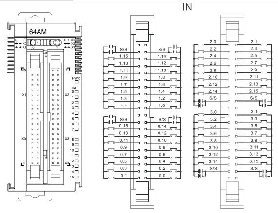
Wiring the External Terminal Module UB-10-ID16A
