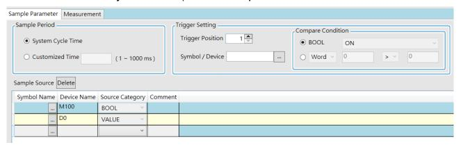
• Click the button of **Symbol Name** in the **Add Sample Source** window and select the variable symbol name to be added in the **Choose Symbol** window or directly type a device name in the **Device Name** box.
