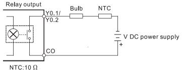
A bulb (neon lamp) is used as an AC load. A thermistor is connected in series to absorb the surge current that occurs when the load is ON.
