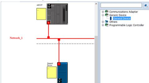
2. Click slave icon and set up its IP address and then configure the parameters in the EIP Parameter tab.
