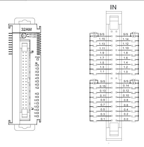
Wiring the External Terminal Module UB-10-ID16A
