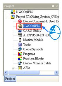
In the **HWCONFIG** window, the default setting is for a CPU module. Refer to Chapter 8 for more information on settings for other types of modules.
