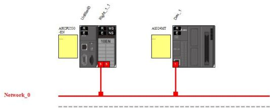
(c) Once the connection is established, click the network line "Network\_0" to see all the connected devices in this network in the Information window.
