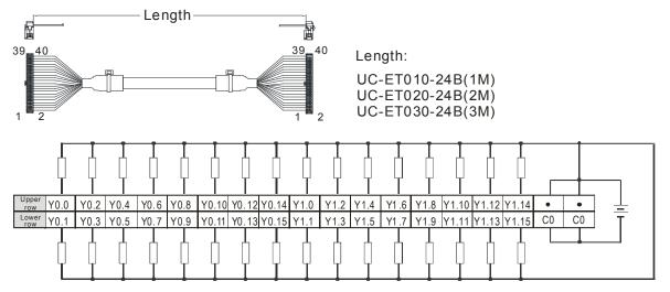
Note: UB-10-OT32A can be used with AS Series and DVP Series. The indications on the UB-10-OT32A board is for DVP Series. For the definitions of terminal connections for AS Series, you can see the reference table below. Or refer to the enclosed sticker for AS Series.
