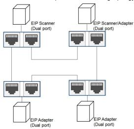
When a switch is needed for topology, the switch should support the DLR function. If not, the connection might fall
