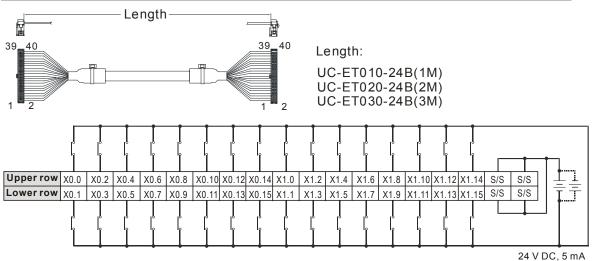
Note: UB-10-ID32A can be used with AS Series and DVP Series. The indications on the UB-10-ID32A board is for DVP Series. For the definitions of terminal connections for AS Series, you can see the reference table below. Or refer to the enclosed sticker for AS Series.
