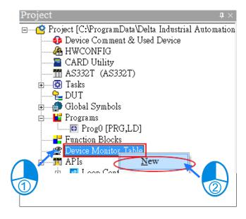
Type a table name in the **Add Monitor Table** dialog box, and then click **OK**. An item appears under **Device Monitor Table** in the project management area. Double-click the item to open the monitoring table. You can create several monitoring tables in the project, and the monitoring tables are saved with the project.
