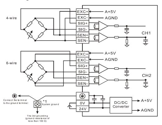
• Multiple load cells connected to one load cell module:
