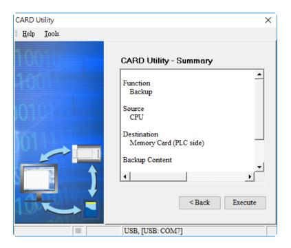
(6) The AS Series CPU module still performs the data backup even if you click Cancel. You can turn off the AS Series CPU module to stop the data backup; however, the backup file produced is not a complete backup file, and you must delete the backup file from the memory card.
