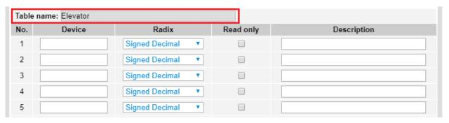
d. Edit the devices to be monitored, radix to be shown, read only or not and the description. After editing, click "Apply" to save the setting.
