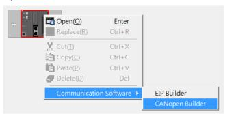
B. IF AS300 is in master mode, you can skip this step. If not, you can go to Properites and set it in Master mode. After that download the parameter to AS300. Set AS300 Power off for 2 seconds and supply power again and then proceed to the next step.
