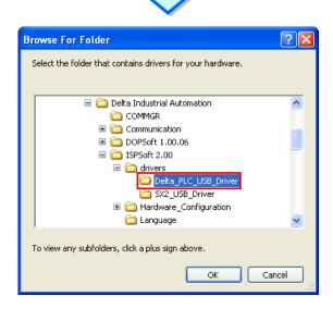
(4) The system installs the driver. If the **Hardware Installation** message appears during the installation, click **Continue Anyway**.
