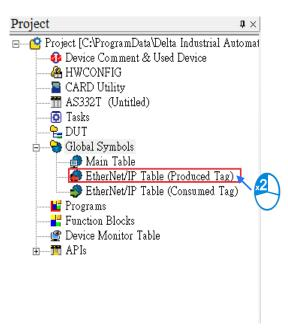
2. Double-click EtherNet/IP Table (Produced TAG) to create a Produced TAG.
