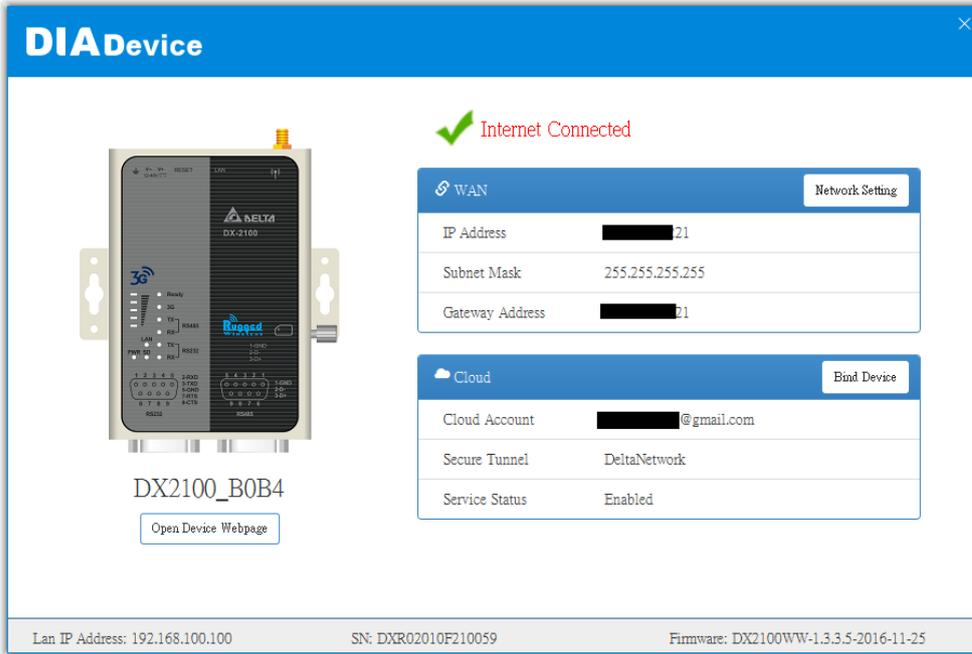
The screenshot shows the DIA Device configuration interface. On the left is an image of a DELTA DX-2100 device with the label "DX2100\_BOB4" and a button "Open Device Webpage". On the right, there are two configuration panels:
