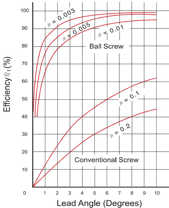
Normal usage (to convert rotary motion to linear motion)
