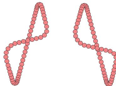
Fig 1.1.4 Internal Ball Circulation Nuts
