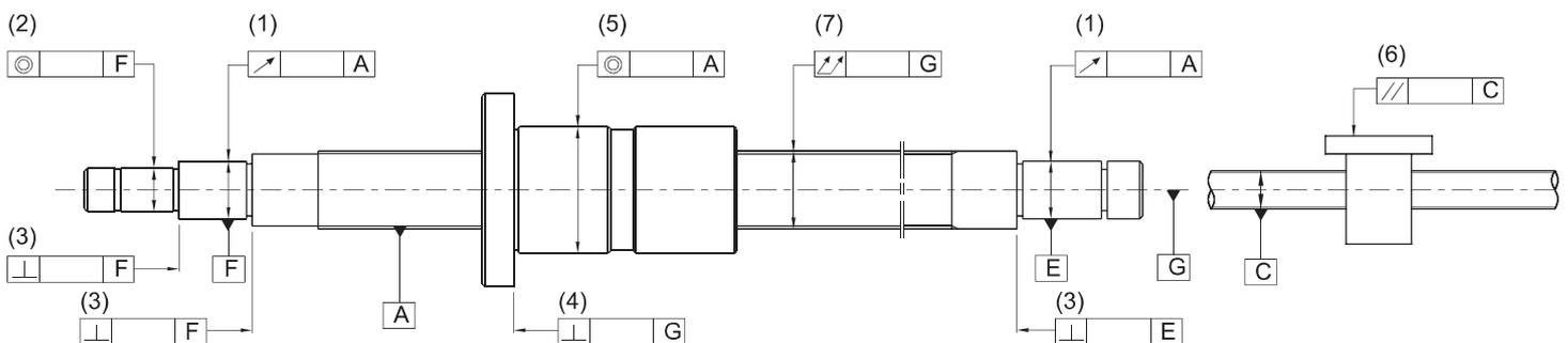
Fig 1.3.2 Mounting Accuracy and Tolerance
