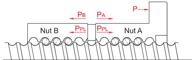
Fig 1.7.1 Preloaded for the double nuts
