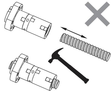
Fig 1.10.1 Error installation
