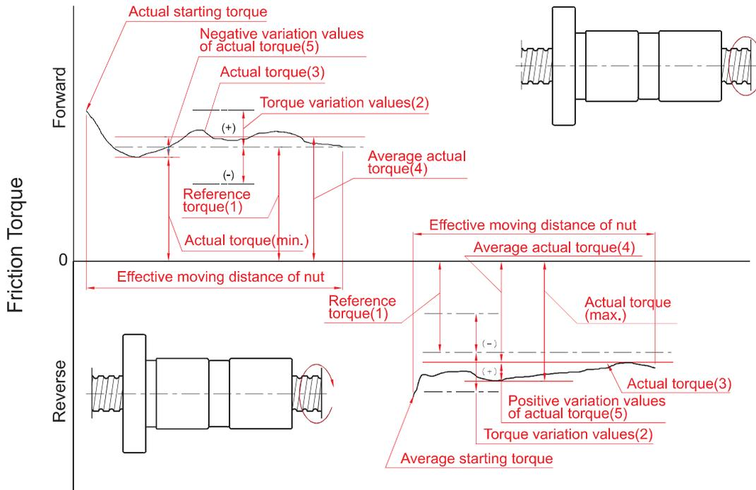
Fig 1.3.3 Descriptions of preload torque
