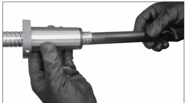
(4) Ensure that the ball nut is fully inserted before remove the mandrel.
