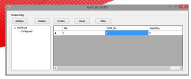
Net: it is same to the Net ID set in the former serial port configuration window.
