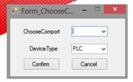
3. choose the com port no. between PC and PLC, the device type please select PLC, then click confirm. Then back to main window, click Config/single device/com port.
