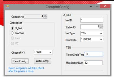
NetID: the network no. of the two PLC. The network no. must be same for the same network, here it is set to 1.
