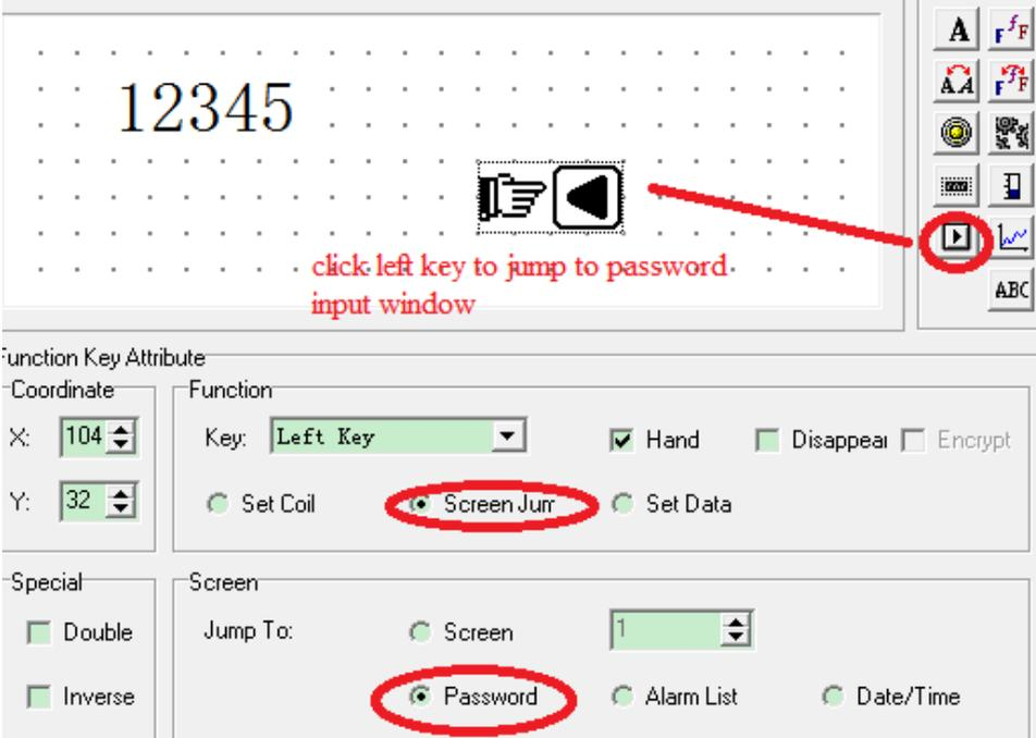
The image shows a control panel interface. At the top, there is a numeric keypad with the digits '12345' displayed. To the right of the keypad is a function key icon (a hand pointing to a left arrow) and a red arrow pointing to a function key icon in the top right corner of the panel. Below the keypad, there is a red text annotation: "click left key to jump to password input window".
