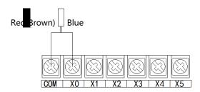
two wires (normally open/closed) proximity switch wiring example
