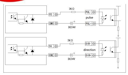
(make sure the current of servo driver optical coupling input is 8~15mA)
