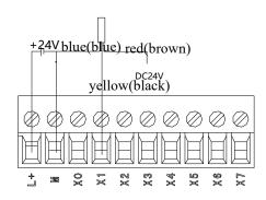
Three wires proximity (NPN) switch wiring
