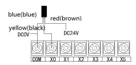
Three wires (NPN) proximity switch wiring example
