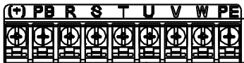
Figure 3-5 3PH terminals of main circuit (220V, \le 0.75kW , and 380V, \le 2.2kW )
