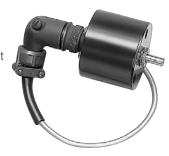
provide smooth control of unwind stands operating at any speed. The sensor is mounted at one end of the dancer roll pivot shaft where it monitors the angular position, direction of travel and relative speed of dancer arm movement. TCS-605-2 used with drive systems.
